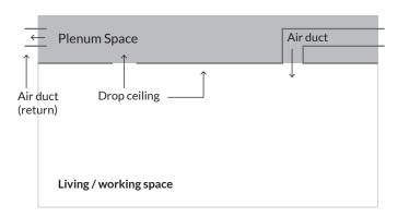
Plenum spaces are the open spaces above the ceiling or below the floor that are used for air circulation. Any cable that you run through plenum spaces must be plenum rated.
